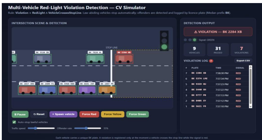
Fig 6. Simulation with Violation and Detect License Vehicle Plate
